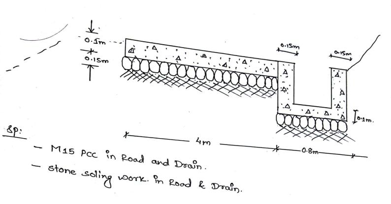
Fig: Typical cross-section of Road Pcc.
